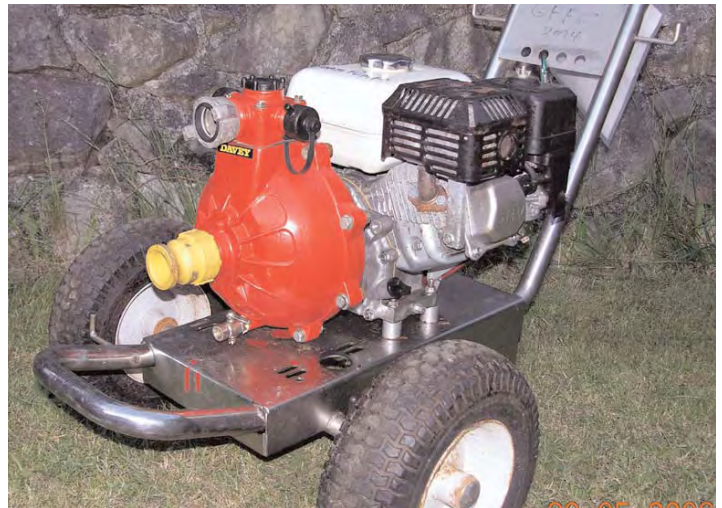
Davey Pump OTS-93216C by Gormann Rupp with a Honda 6.5hp engine. Pumps 66gpm and develops 360ft of head = 156psi List price $2,500 without mounts
