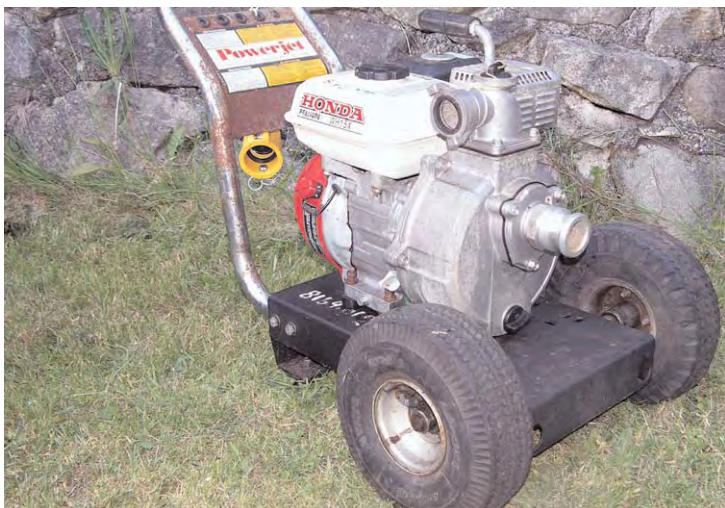
The Honda WH15x pump is a good draught pump. With a 4hp engine it pumps 115gpm US and develops 164ft of head = 71psi. List price $769 without frame or wheels
