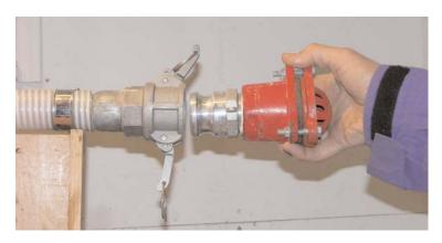
To connect our GFEG pumps to well intakes and tank fittings, all your intakes have been modified to include quick-release fittings. They consist of camlock couplings between the red foot valves and the flexible intake hose. The intake (left) disconnects from the red foot valve (right). It can then be connected to the camlock adapter on the well or tank (above). This is a fast easy coupling that could make a big difference when time is of the essence.
